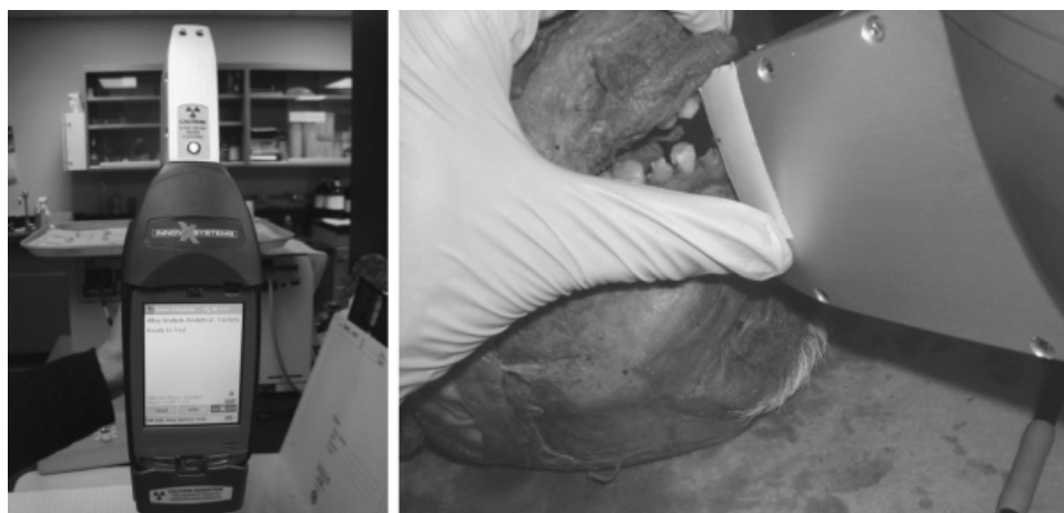
FIG. 3—Portable X-ray fluorescence in use to locate and identify resins in situ.
